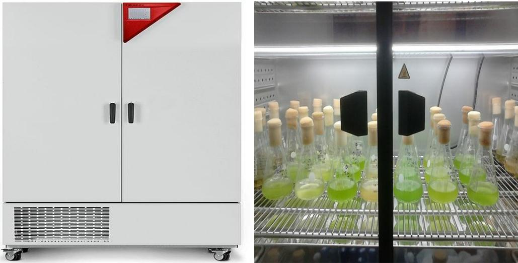
Figure 4. Binder reach-in growth chamber for R&D optimisation and small-scale cultivation.
